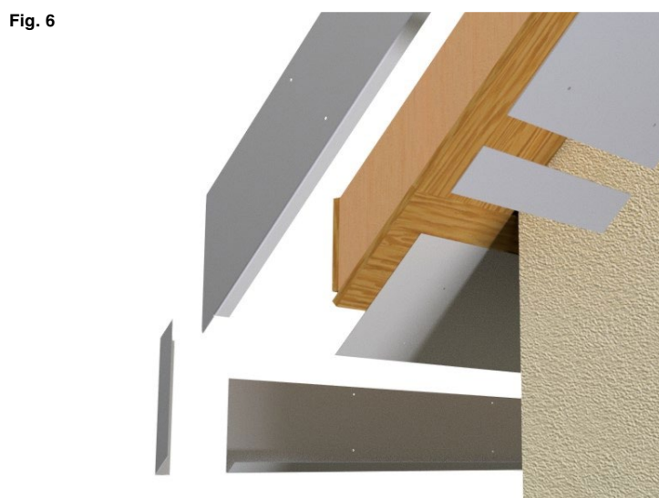
Angled soffit box end construction
